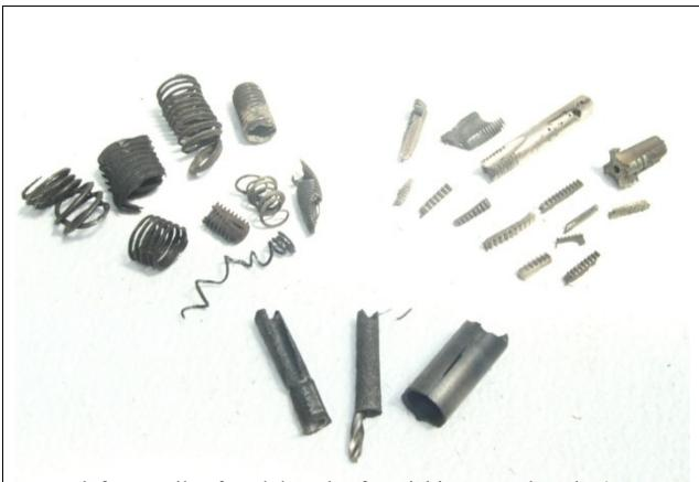
Upper left are coils of stud threads after picking out. They don't usually come out in one piece as this might imply.
