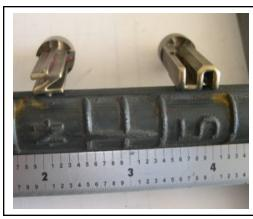
Rebar roller die was engraved with EDM Electrode letters are brass. Roller die not shown.
