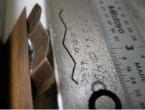
Electrode is .006 copper. Slot is .013 wide .040 deep Zigzag electrode is stiffer than flat electrode.
