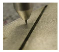
Job: Cut slot 1 mm wide x 30 mm long 1 mm deep in steel for calibration of ultrasonic crack testing calibration. Electrode: Graphite Time: 6 minutes
