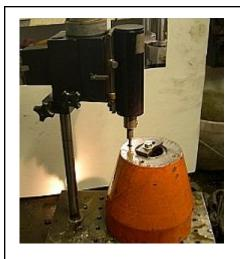
Job: Remove 5/16-18 Broken tap from casting.
