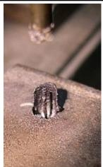
Remove 3/32 dowel pin. Electrode .072" Brass tubing Time = 3 minutes.
