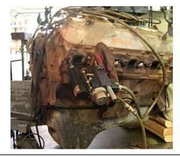
Setup on exhaust stud in V8 Motor
