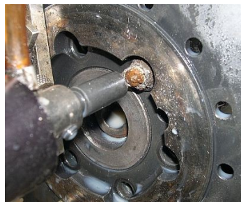
Job: Broken stud in crankshaft end plate. Engine is in vehicle and on a lift with transmission and flywheel removed (photo 1). Machine is set up using a neighbor threaded hole in crankshaft (photo 2). Hole after EDM work and before picking out remaining thread sleeve Electrode: Graphite tube 10 mm stud 20 mm deep Time: 12 minutes. Last photo shows stud removed and ready to pick out remainder of thread sleeve .
