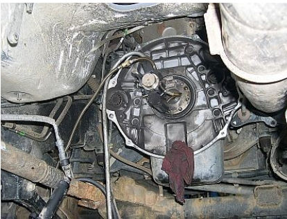
Job: Broken stud in crankshaft end plate. Engine is in vehicle and on a lift with transmission and flywheel removed (photo 1). Machine is set up using a neighbor threaded hole in crankshaft (photo 2). Hole after EDM work and before picking out remaining thread sleeve Electrode: Graphite tube 10 mm stud 20 mm deep Time: 12 minutes. Last photo shows stud removed and ready to pick out remainder of thread sleeve .
