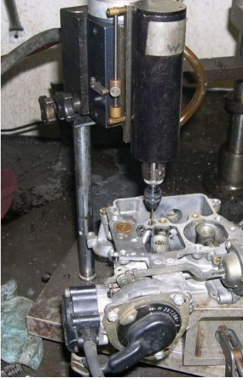
Carburetor with small needle valve screw to be removed. Electrode: .062" Brass tubing. Time: 2 min-
