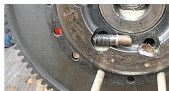
Job: EDM stripped head of ring gear bolt. Then unscrew bolt by hand. Again, working under lift. Rear of engine shown. Electrode Graphite Tube 5/8 OD x 3/8 ID Time = 6 minutes
