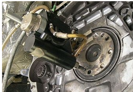
Job: Broken stud in crankshaft end plate. Engine is in vehicle and on a lift with transmission and flywheel removed (photo 1). Machine is set up using a neighbor threaded hole in crankshaft (photo 2). Hole after EDM work and before picking out remaining thread sleeve Electrode: Graphite tube 10 mm stud 20 mm deep Time: 12 minutes. Last photo shows stud removed and ready to pick out remainder of thread sleeve .
