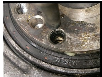
Job: Broken stud in crankshaft end plate. Engine is in vehicle and on a lift with transmission and flywheel removed (photo 1). Machine is set up using a neighbor threaded hole in crankshaft (photo 2). Hole after EDM work and before picking out remaining thread sleeve Electrode: Graphite tube 10 mm stud 20 mm deep Time: 12 minutes. Last photo shows stud removed and ready to pick out remainder of thread sleeve .
